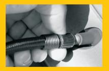
Screw connector on air valve stem
