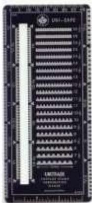
One of the simplest and most important factors in identifying and valuing a stamp is determining its Perf. This sturdy perforation-gauge with cutout inside gauge to allow for easy matching of mounted stamps. In addition to perforation gauge, includes inches and millimeter measurements.
